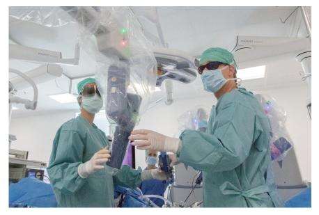
The Senhance Surgical System is the only commercially available robotic surgery system with haptic feedback, a differentiating feature for surgeons.
